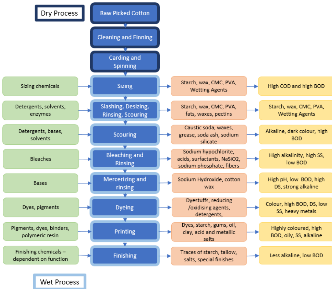
Figure 13: Process diagram showing the difference in input (green), output (orange) and wastewater characteristics (yellow) for each of the steps (blue) in the textile industry. The figure was amended from process diagrams by (Dey & Islam, 2015; Mia et al., 2019)
