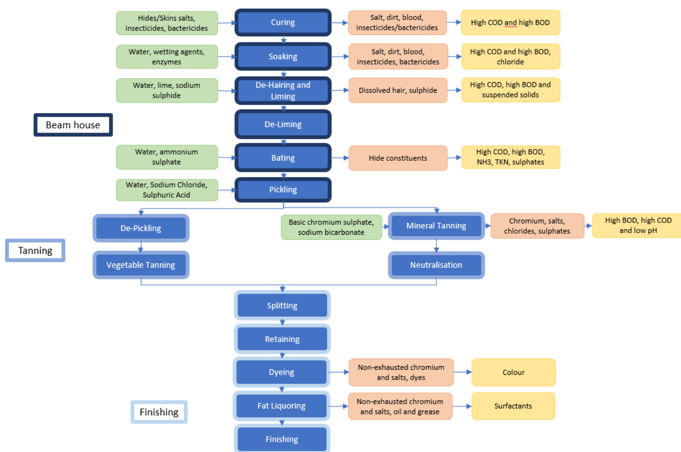
Figure 11 Process diagram for different stages of leather production, showing the input (green), output (orange) and typical effluent characteristics (yellow) from each process (blue). This figure was amended from information from (A. Hoque & Clarke, 2013)
