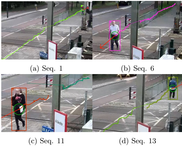
Figure 14: Successful (a, b) and unsuccessful (c, d) handling of occluded part in track.
