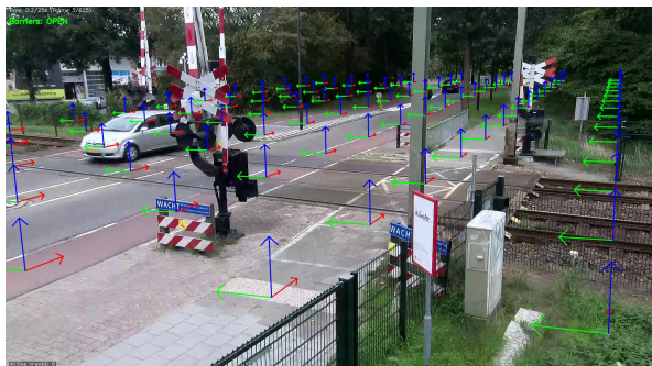
Figure 6: Extrinsic camera parameters established by providing a rough estimation and subsequently using the known height of person detections to fit a more accurate model. Visualized by a grid of orthonormal direction arrows on the ground plane in world space.
