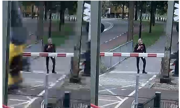
Figure 10: Video compression artifacts. Left: a train just passed by. Right: image quality stabilized after a second or two.
