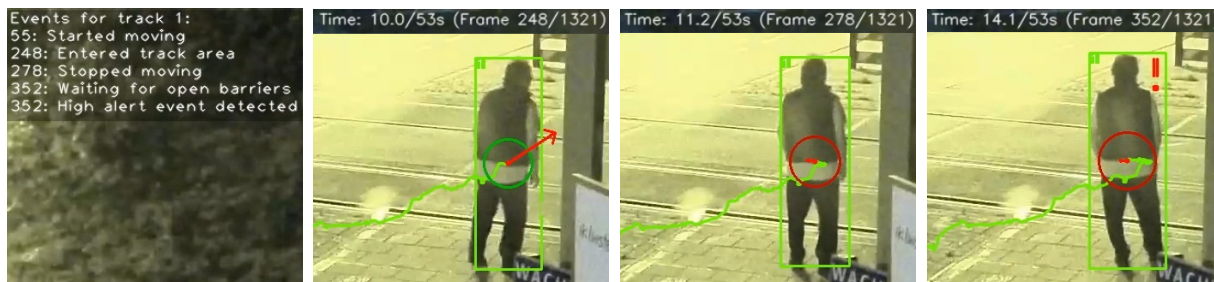
(a) Detected events with frame number. (b) Person appears to stop moving. (c) Stop event is detected. (d) 3 seconds after the person was detected to have stopped moving an alert was triggered because the barriers were open.
