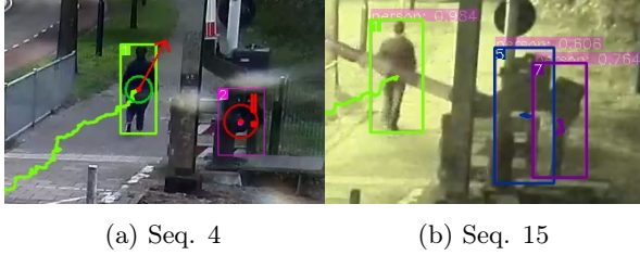
Figure 13: False alarm tracks. FAT in (a) persists long enough to trigger an alert for waiting while barriers are open.
