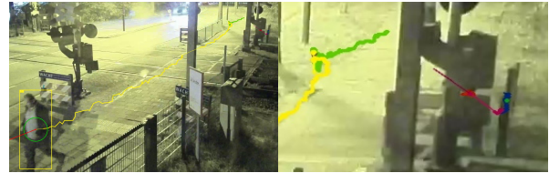
Figure 12: One track fragmentation due to train passing by and several false alarm tracks (seq. 16).
