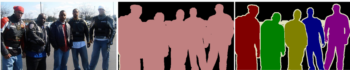
Figure 1.1: Example annotations for segmentation tasks, taken from the Pascal VOC dataset [14]
