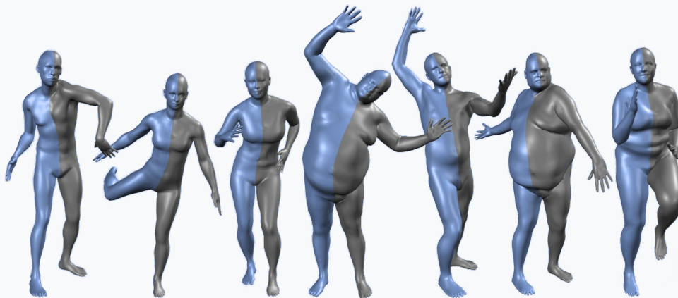
Figure 2.7: Examples of SMPL model fits to a limited number of keypoints (blue) and full ground truth poses (grey). Figure adapted from [55].
