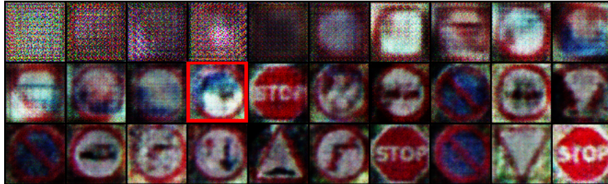
Figure 7: Visualization of the GAN training progress over 30 epochs. Starting in the top left corner (and moving along the row), each image represents one training epoch. The threshold of 30% accuracy is reached after 14 epochs (highlighted in red).
