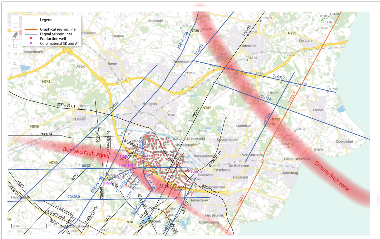
Figure 5: Locations and spatial distribution of subsurface data in relation to the approximate location of the fault zones. Background map from (NLOG, n.d.) location of the faultzones after figure 12.5 from NITG-TNO (1998).
