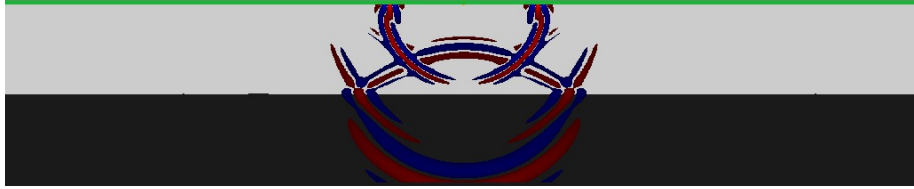
Figure 9: Snapshot of the model with one reflector at t=3600 msec: two layer model, particle velocity.
