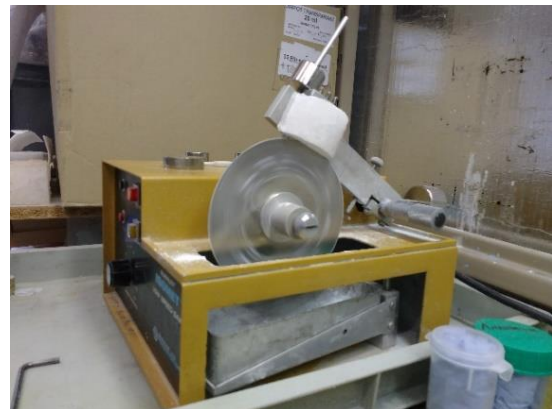
Figure A.3: Making the thin sections of the sample using the diamond wafering blade, which cleans itself by rotating in the evaporating oil filled container at the bottom of the apparatus.
