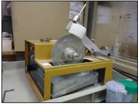
Figure 15: Making the thin sections of the sample using the diamond wafering blade, which cleans itself by rotating in the evaporating oil filled container at the bottom of the apparatus.
