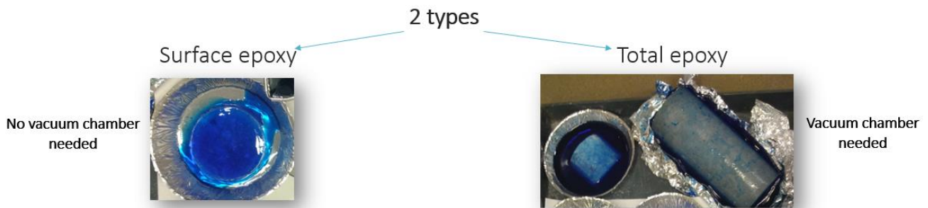
Figure A.2: Two ways to apply epoxy on your sample: surface epoxy and total epoxy.
