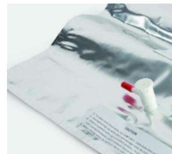
Figure 7: Multi-Layer Foil Gas Sampling Bag. Source: https://www.restek.com/catalog/view/11097 .
