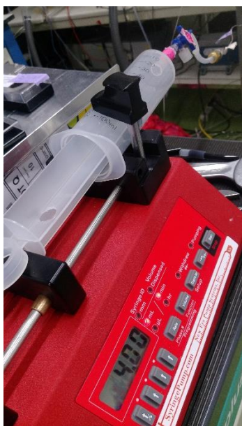
Figure 20: Syringe pump. Picture taken by Caroline Jacques.
