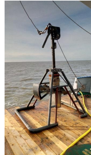
Figure 11: Box corer on board of the Navicula. Picture taken by Julia Engelmann.
