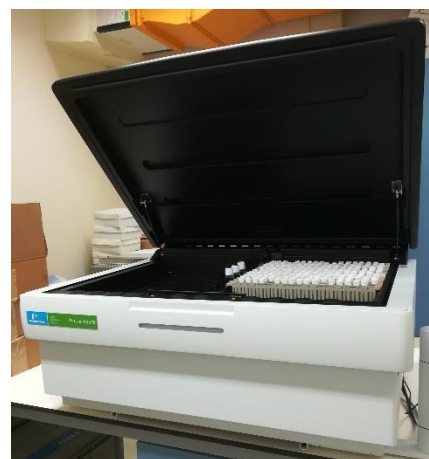
Figure 13: TRI-CARB 4810TR Liquid Scintillation Counter at NIOZ Texel containing water samples from the autumn cruise.
