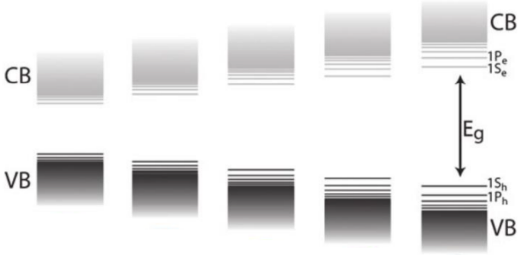
Figure 2.4: A graphical representation of the change in band structure when decreasing the size of the crystal. Left is the band structure for bulk material, moving to the right corresponds to a smaller crystal size. Adapted from ref 6
