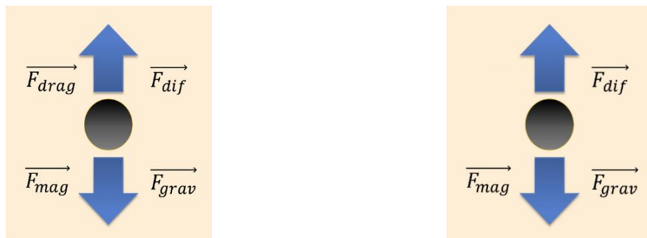
Figure 3: Left: Forces on a sedimenting superparamagnetic nanoparticle, right: Forces on superparamagnetic nanoparticle at sedimentation-diffusion equilibrium
