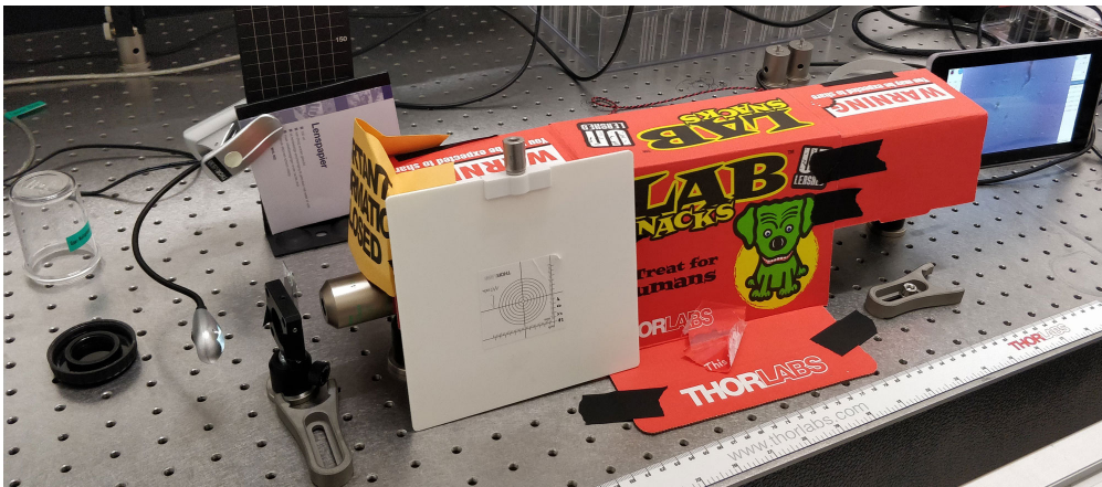
Figure 2.7: Setup used for trans-illumination with a continuous light source.
