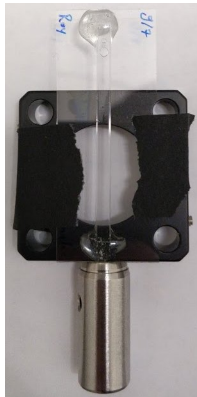
Figure 2.3: Attachment of the capillary containing the emulsion to an optical cage.
