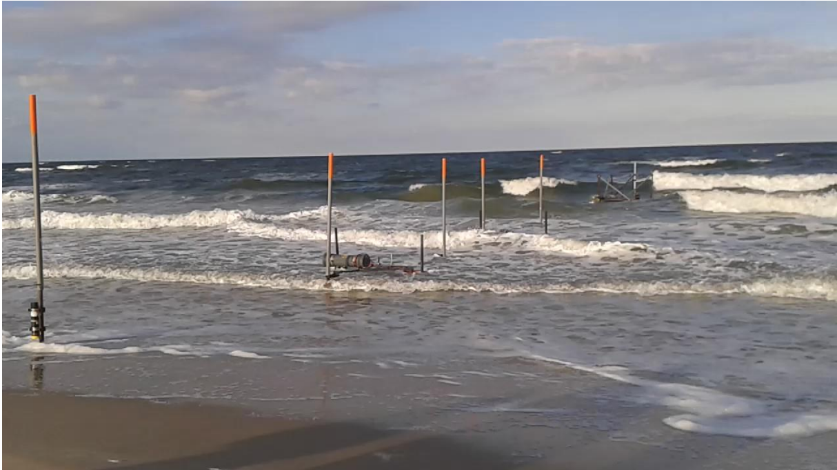
Figure 3.1: Photograph of the setup of some of the instruments deployed in the transect. Taken during high water in the morning of 23 th of September during moderate energetic wave conditions. From left to right: OSSI 5, miniframe 15, OSSI 4, miniframe 13, OSSI 3 and CRD. OSSI 2 and OSSI 1, also part of this frame transect, are completely inundated and thus not visible in this photo.
