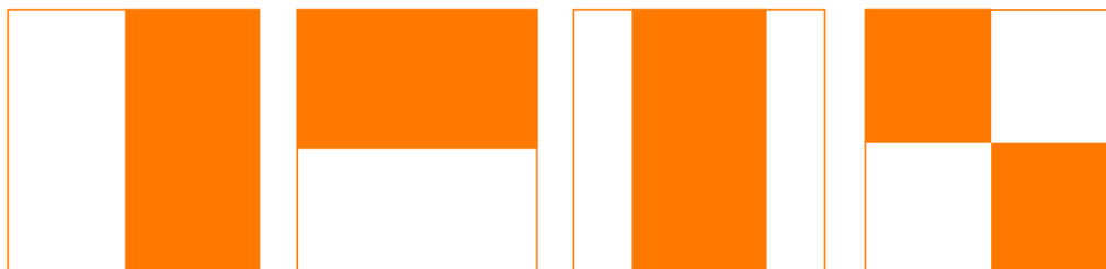
Figure 2.4: Haar-like features: (1) and (2) Edge features; (3) Line feature; (4) Four-rectangle feature.
