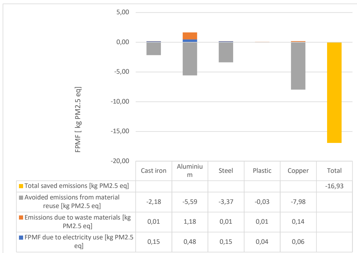
Figure 20 – FPMF Diesel genset recycling
