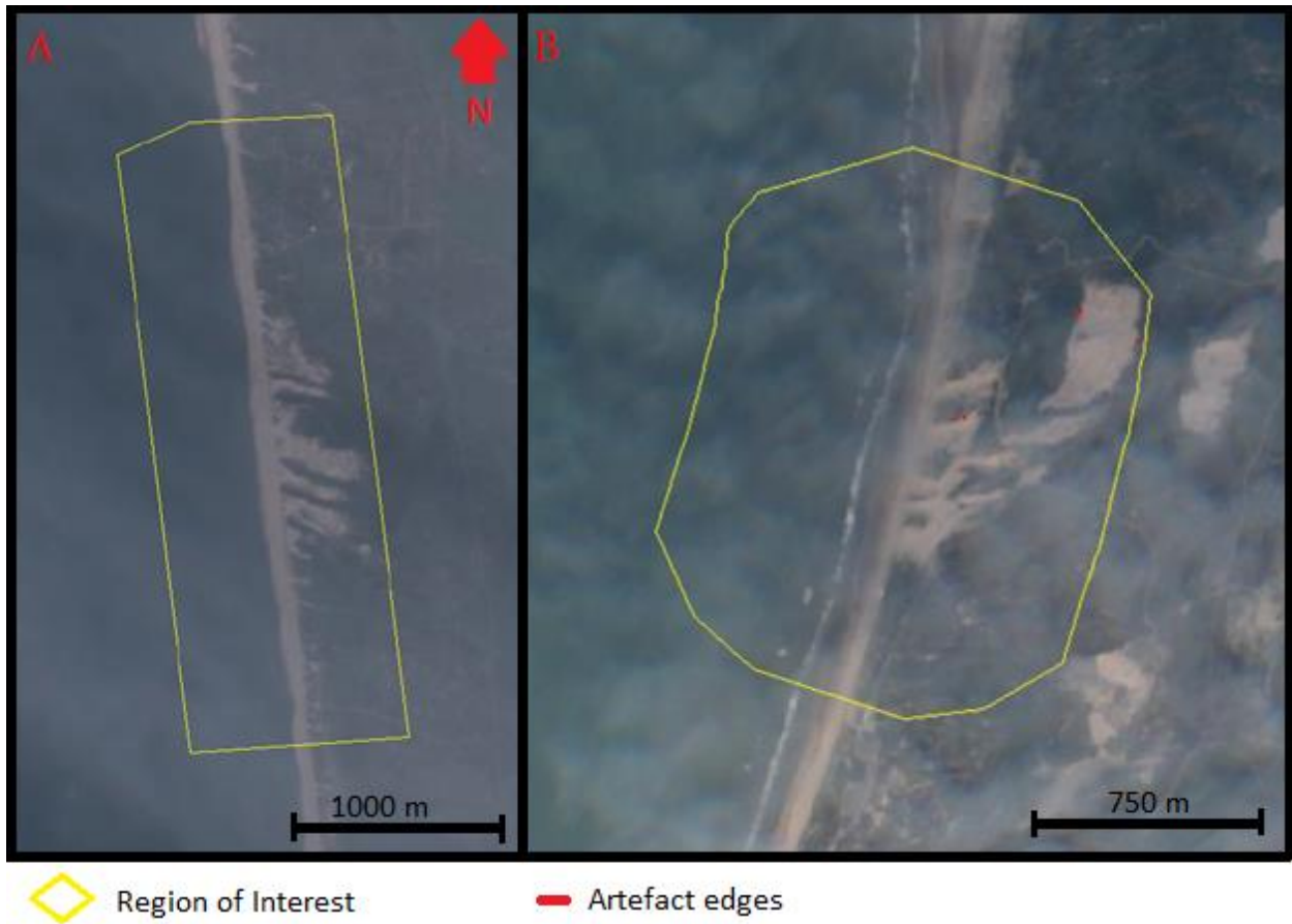
Figure A-8; Sentinel-2 images of A) Haurvig (2015-09-11) and B) Zuid-Kennemerland (2015-08-05) in true colour. The yellow line represents the ROI for each study site. No edges were detected in image A, while only suppressed, short segments of connected edges were detected in image B (red pixels).
