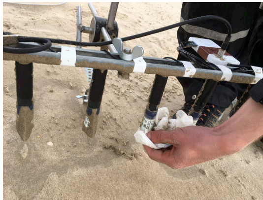
FIGURE 3.7: Impact sensors being wiped clean after having become clogged with sticky wet sand during a period of intense rainfall.
