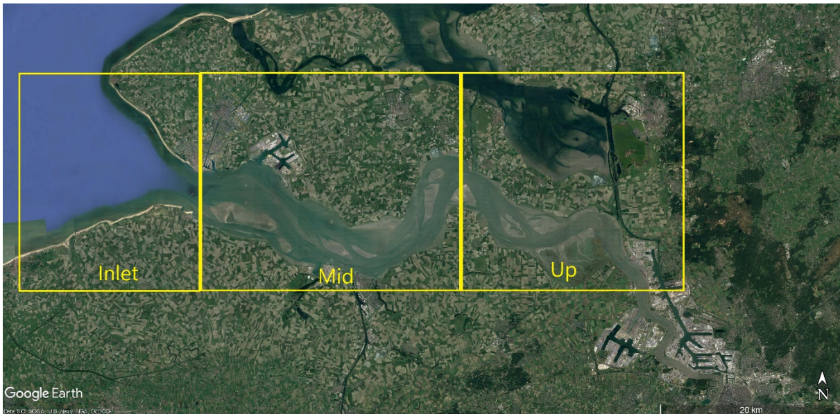
Figure 4 Sections of the Western Scheldt estuary (Google Earth, 2019). The Inlet section is characterised by a large estuary volume, modelled as infinite (e.g. the sea). For the mid- and upstream sections is the water volume calculated based on the area of the estuary.
