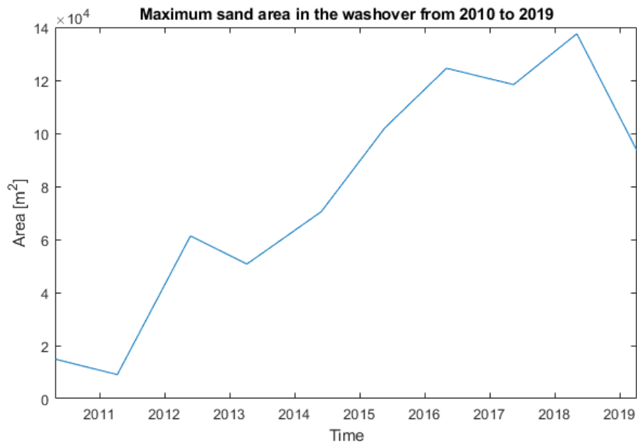
Figure 4.9. The evolution of the maximum sand area in the washover. The maximum sand area is the maximum surface area of the sand inside the washover for a year, which is assumed to be an indication for the size of the washover.
