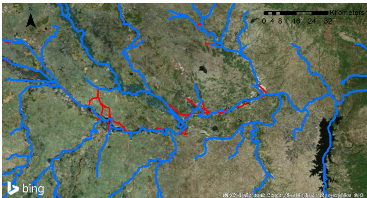
Figure 5: The red lines show the old river flow path; the blue lines show the river flow path after adjusting the DEM. The backdrop is an aerial photo showing the rivers actual flow path (Bing Maps Aerial, 2019).
