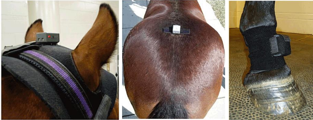
Fig. 1: A horse instrumented with the Lameness Locator system of Equinosis®, whereby accelerometers are placed on the head, pelvis and the pastern of the right front leg (McCracken, Kramer et al. 2012)
