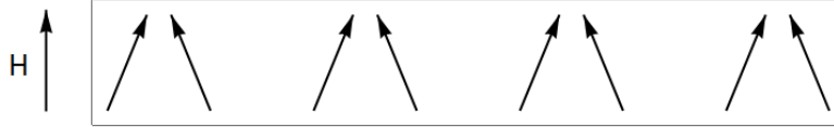
Figure 3.3: Graphical depiction of a antiferromagnetic state when the magnetic field is above the spin flop field ( h > h_0 ).
