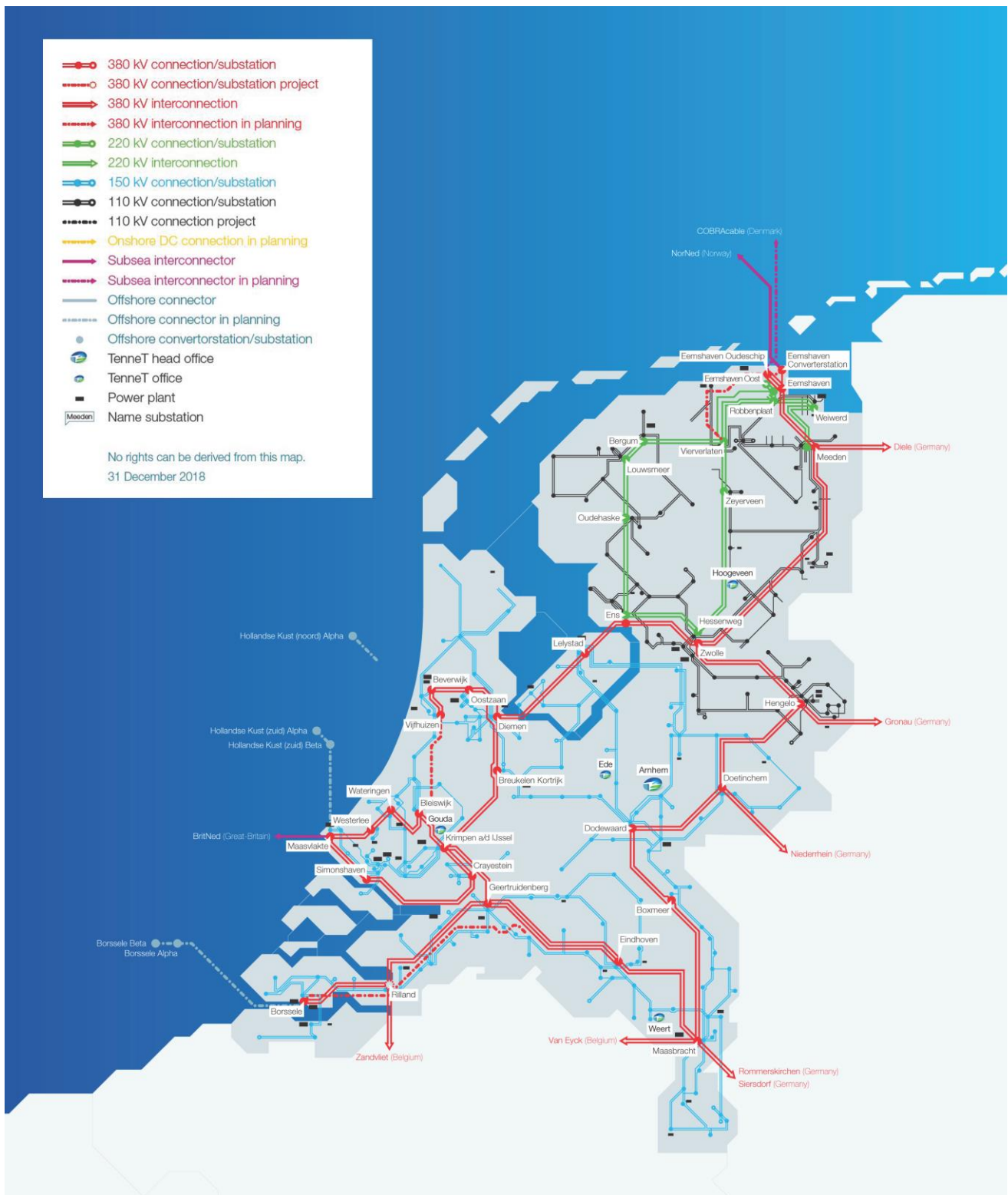
Figure 2.3: The Dutch (extra) high voltage grid (380, 220, 150 & 110 kV) (TenneT, 2018)
