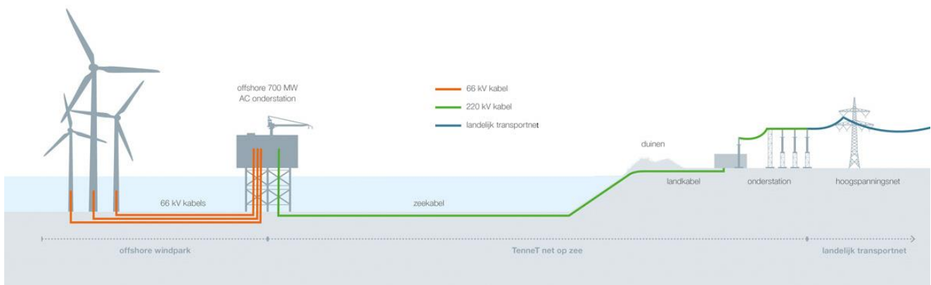
Figure 2.14: Schematic illustration of a grid connection for an offshore wind park (Noordzeeloket, n.d.)
