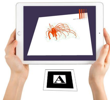
Figure 3.4: Flow map concept in a MR environment. The map is perceived on an iPad, aimed at the target on a flat surface such as a table.
