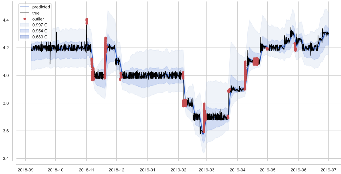
Figure 7.13: Quantile plot of sensor 104OYE, with added jump using the univariate perceptron model.
