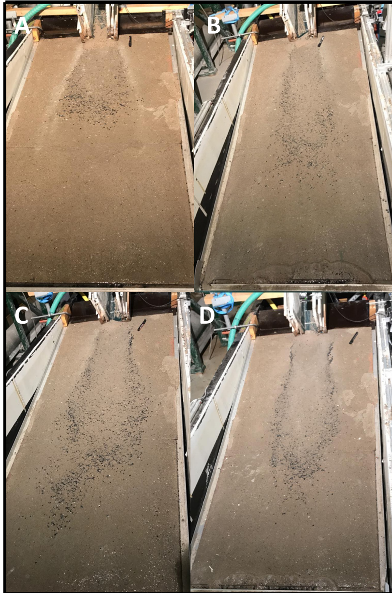
Figure 4.18. Subaqueous debris flow deposits with varied outflow channel slope A) Slope 20^{\circ} , B) Slope 25^{\circ} , C) Slope 35^{\circ} , D) Slope 40^{\circ} .
