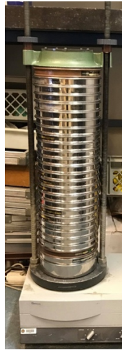
Figure 3.4: Complete order of sieves, performing sieve analysis.
