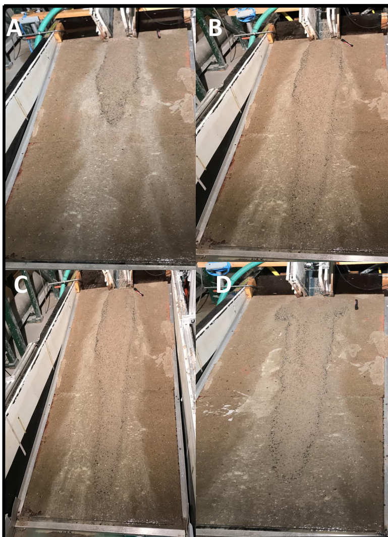
Figure 4.19: Subaerial debris flow deposits with slope variations A) Slope: 20^{\circ} , B) Slope: 25^{\circ} , C) Slope: 35^{\circ} , D) Slope: 40^{\circ} .
