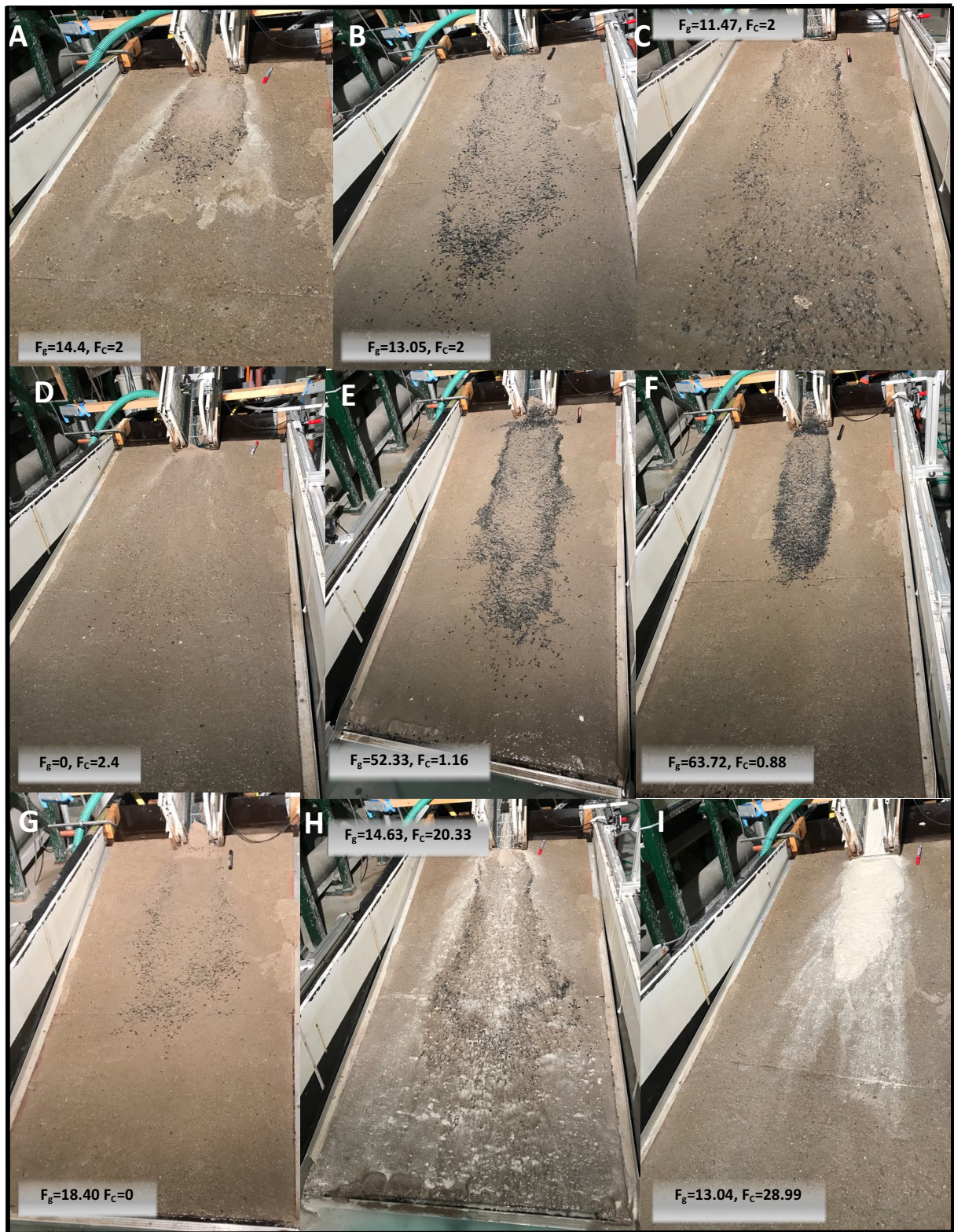
Figure 4.13 Subaqueous debris flow deposits with varied composition A) Water 40%, B) Water 50%, C) Water 60%, D) Gravel 0%, E) Gravel 52 %, F) Gravel 64%, G) Clay 0%, H) Clay 0.11, I) Clay 0.29% content.
