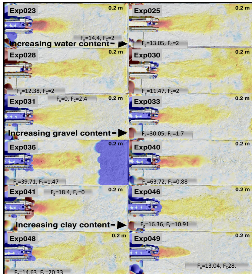
Figure 4.15 DEM Photo-scans of subaqueous debris flow deposits of varied composition, Exp023-Exp030) Water content (volume 40-50 %), Exp031-Exp040) Gravel content (volume 0-64%), Exp041-Exp049) Clay content (volume 0-29%).
