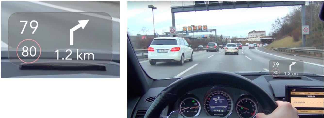
Fig. 5 - HUD interface proposal. The HUD display (right) and what it looks like from the driver's perspective (left).
