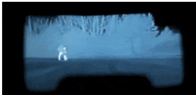
Fig. 4 - Night vision thermal camera applied in HUD interface HUDWAY.
