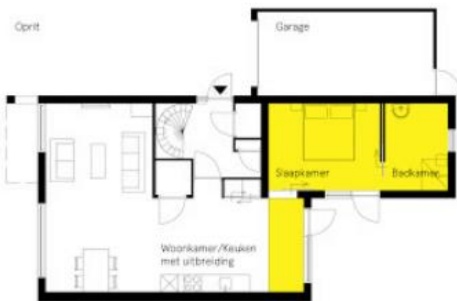
Figure 10b.. Possible home modification, moving the kitchen to create a bedroom and bathroom on the ground floor.
