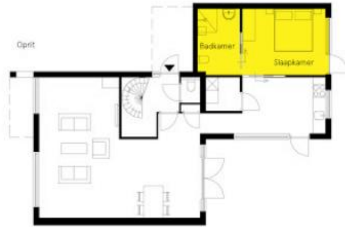
Figure 10c. Possible home modification, creating a bathroom and bedroom out of the garage.
