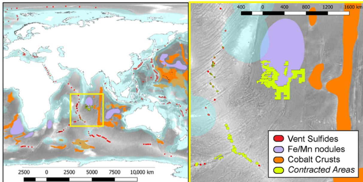
**Figure 4.3** – Superposition of mineral resources and exploration license zones in the central Indian Ocean. Left: global seabed resource distribution. Right: closeup view of yellow bounded box. From Orcutt et al. (2020)
