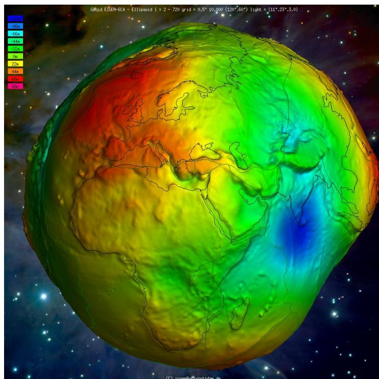
**Figure 2.3** – The Geoid. Undulations are multiplied with a 'boost' factor to enhance visibility (Ince et al., 2019)
