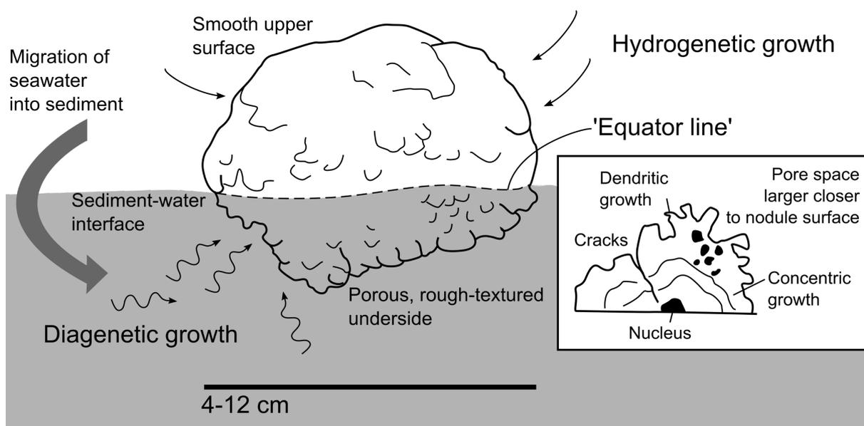
**Figure 3.3** – Schematic illustration of Mn nodule formation and situation at the seabed
