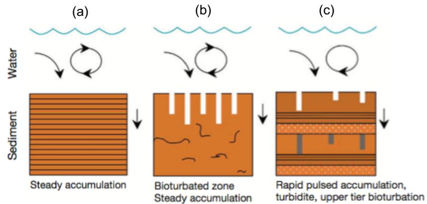
**Figure 2.5** – Benthic transport models. (a) Steady vertical accumulation; (b) steady vertical accumulation with bioturbated surface; (c) episodic sedimentation by turbidites, and stable bioturbation. From Aller (2014)
