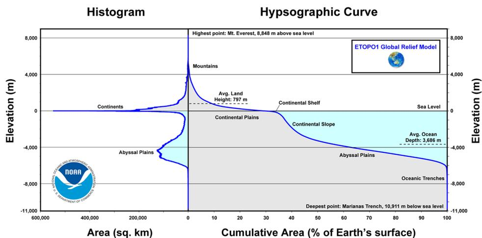
**Figure 2.2** – Global histogram (left) and hypsographic curve (right) of Earth's surface (Eakins and Sharman, 2012)
