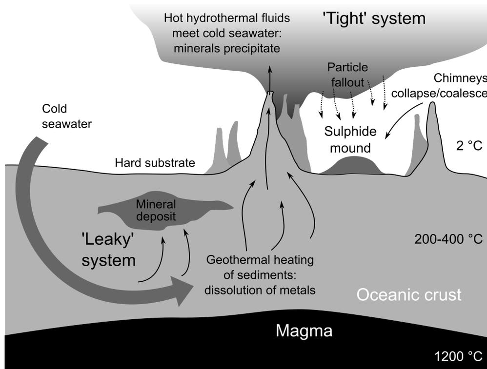
**Figure 3.4** – Schematic illustration of SMS formation and situation at the seabed
