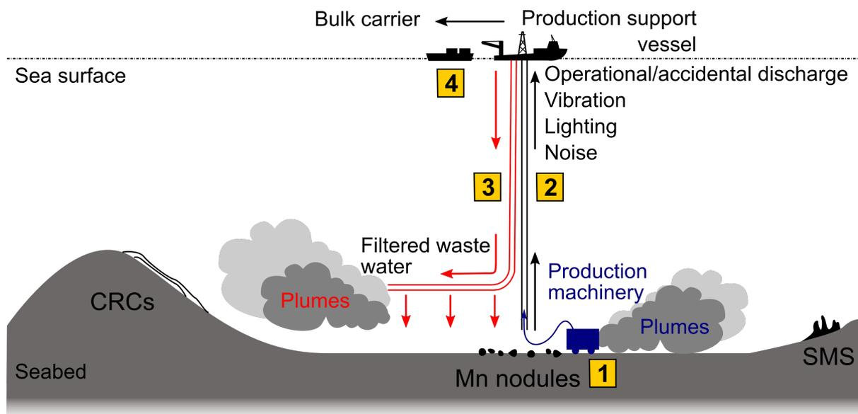
**Figure 3.6** – Stages of SBM operations, corresponding to numbered list above. Modified from SPC (2013a)
