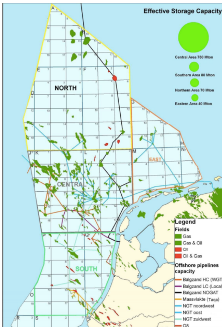
Figure 4.2: Map showing gas fields in the Dutch continental shelf that can be used for storage of CO 2 and the effective storage capacity of certain areas of the Dutch continental shelf
