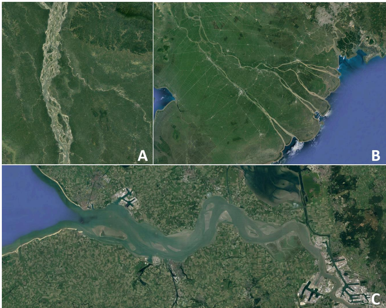
Figure 1.1 Satellite images of fluvial and tidal systems displaying bifurcations and confluences (A, Jamuna. B, Mekong delta. C, Scheldt estuary)
