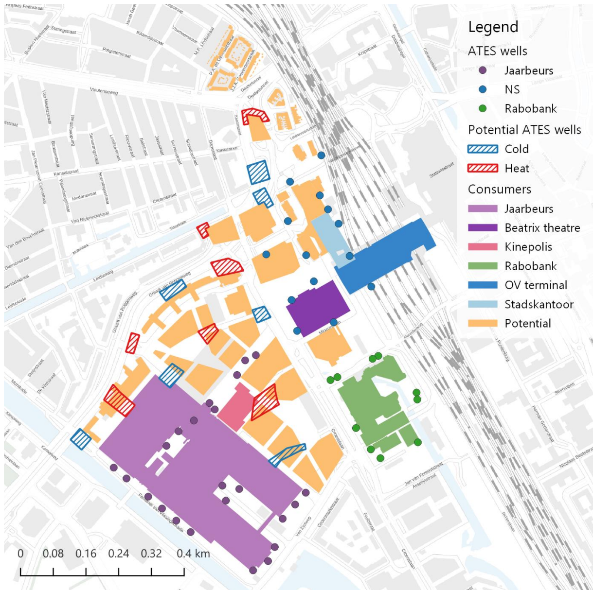
Figure 5 Existing and potential ATES systems
