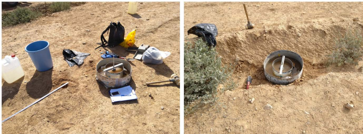
Figure 6 Test site set up of the double-ring infiltrometer. Inside the furrow (right) and on the hillslope (left).
