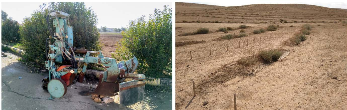
Figure 3 Left: the plough used to create the Vallerani RWH structures. Right: the landscape with the Vallerani RWH structures.
