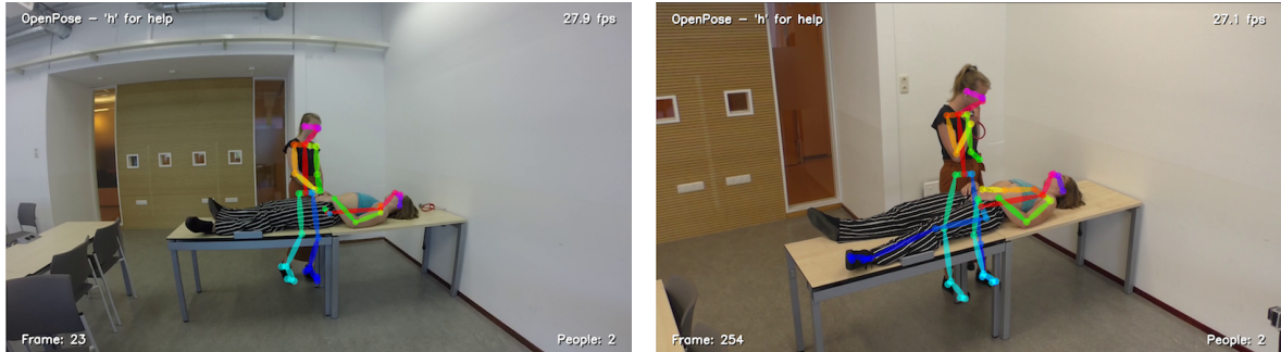
Figure 7.3: Wrongly obtained 2D skeleton for two camera positions. Especially the legs of the patient are difficult to identify. Left: camera, right: GoPro
