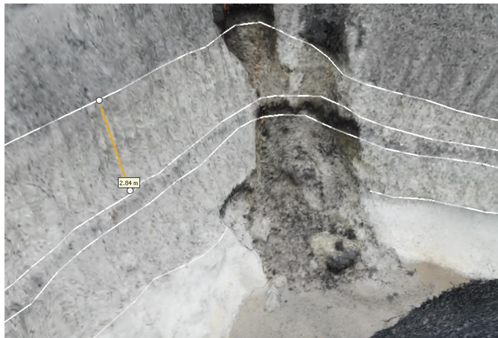
Figure 4.17: Drawing 3D polylines and measuring layer thickness in a DOM.
