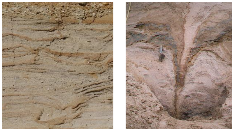
Fig. 2.6 & 2.7: Examples of bedding structures in sand layers (left) and an ice wedge (right). (Source: TNO-GDN, 2019)
