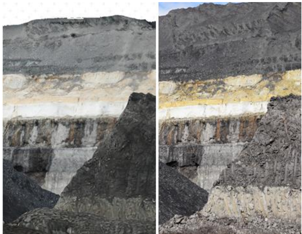
Figure 4.12: DOM level 1 (left) and photograph (right), showing the loss of detail in the DOM.
