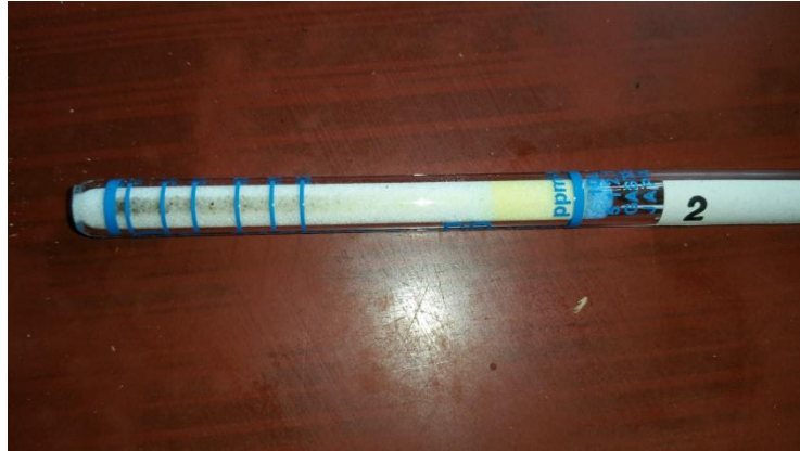
FIGURE 17 AN EXPOSED CO GASTEC DOSITUBE (DISCOLOURATION JUST ABOVE 200PPM*H)
