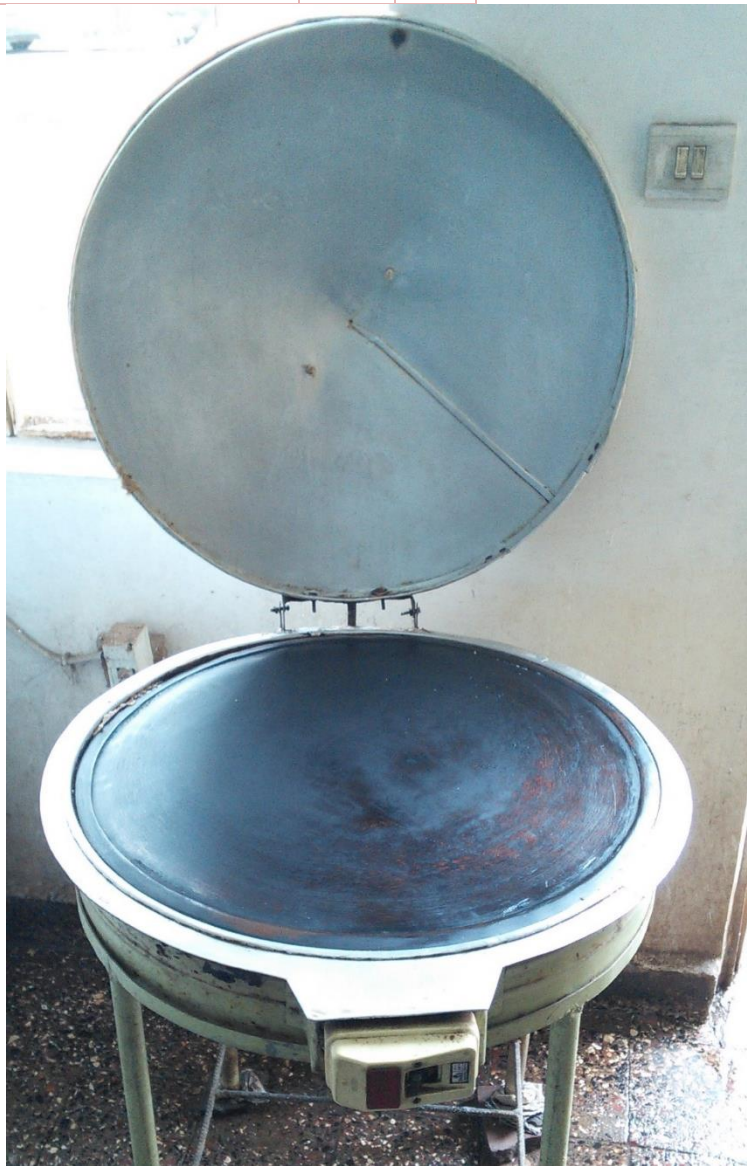
FIGURE 19 EXAMPLE OF A COMMONLY USED ELECTRIC MITAD (Energypedia, 2014)
