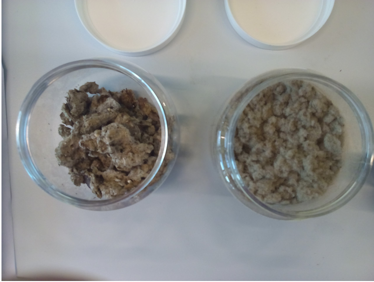
Figure 11 Left: WTP derived from the sludge at WWTP Horstermeer washed and dried. Right: WTP after pulverization in the blender.
