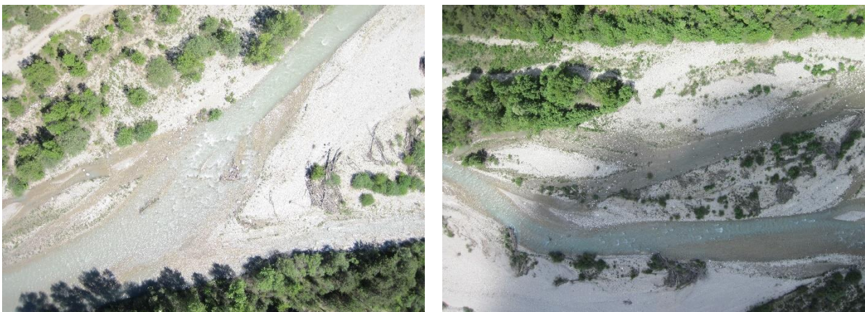
Figure 50 Example of imagery with different lighting. This affects the ability of the program to find common points as the sun is too bright or clouds are temporally covering part of the catchment
