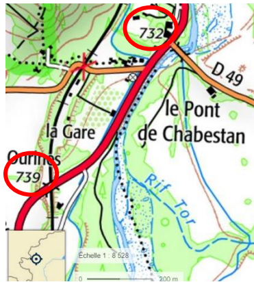
Figure 51 Highlight from the official topographic map of France on their geoportal (height values in the red circle). The values showed are from surrounding areas of the river
