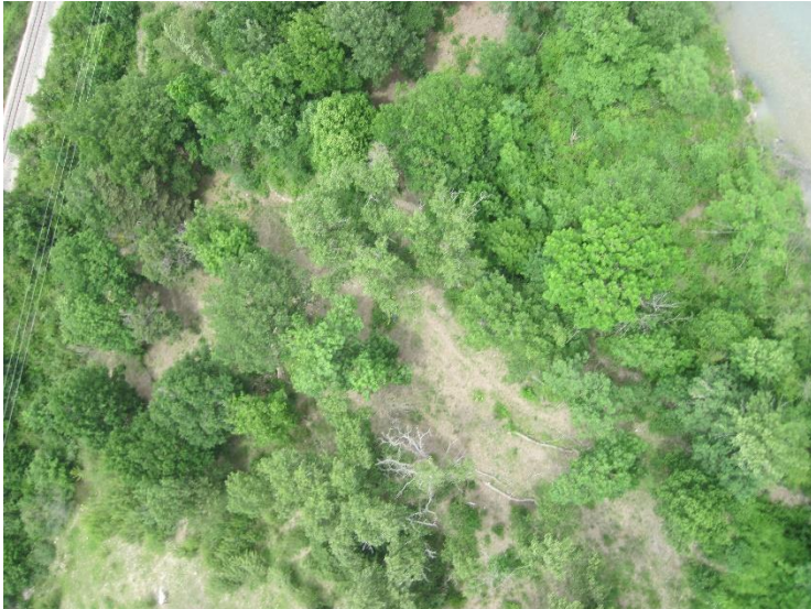
Figure 49 Example of a decent quality photo not usable as the program couldn't align it and find common key points, even with the presence of a still feature as the train tracks
