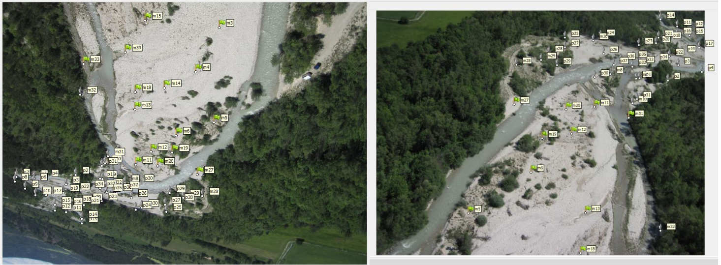
Figure 46 Two examples of decent quality resolution imagery, but bad angles of shooting. The markers in the end of the catchment are impossible to manually locate, returning higher uncertainty and a less accurate alignment
