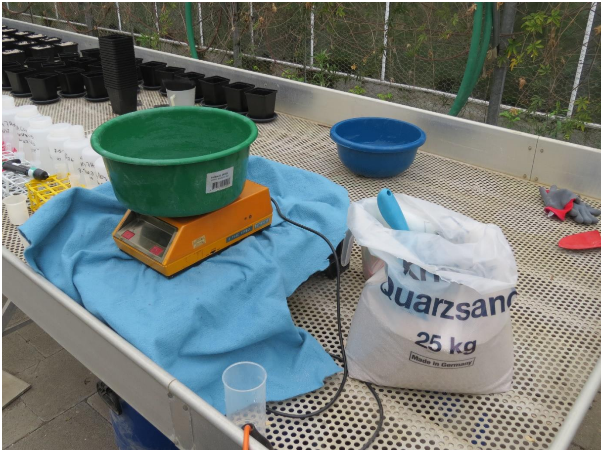
C: Quartz sand from Germany used as main soil component and weighing set-up
