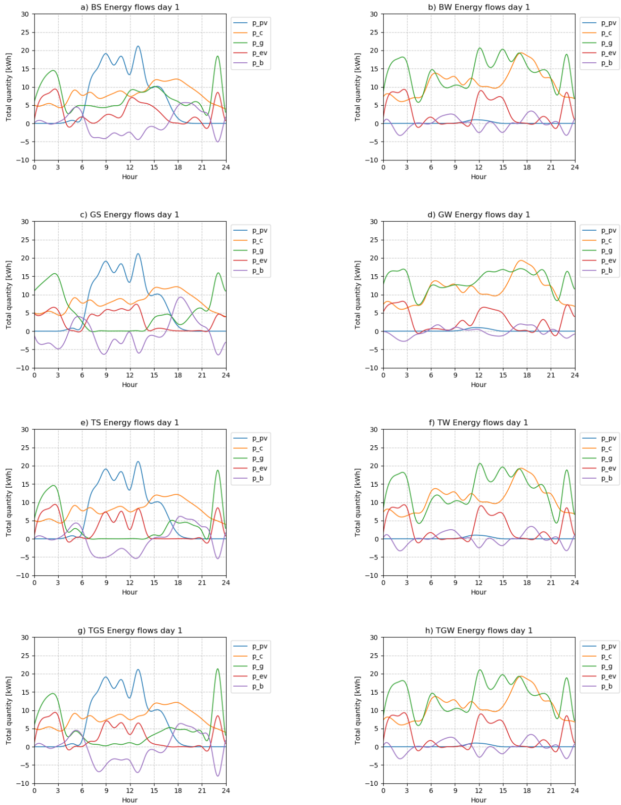
Figure 7: Energy flows for day 1 of the week. All energy flows represent the combined total sum of all households in the community.
