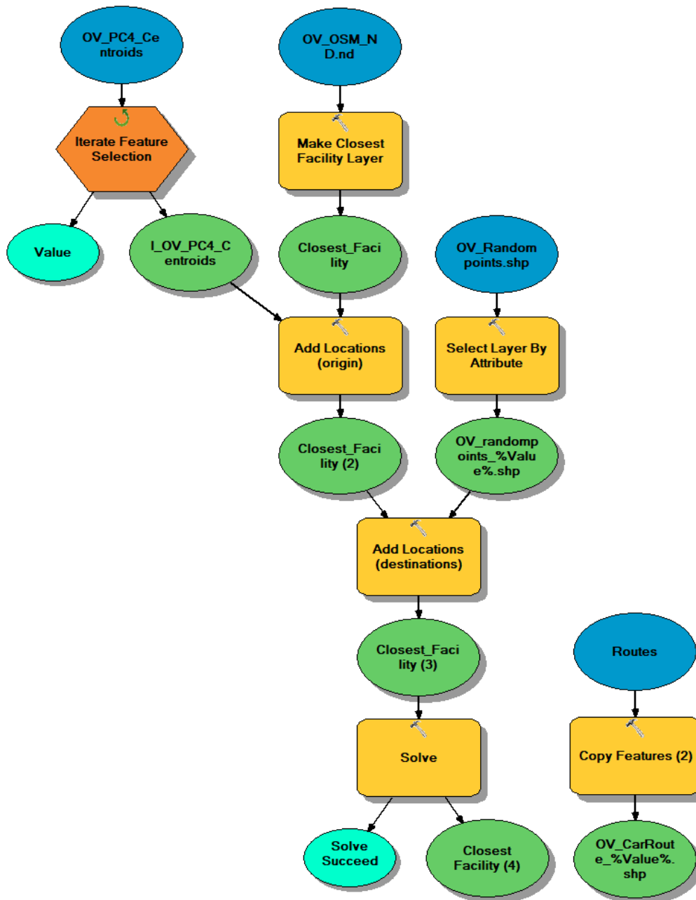
Figure 10: Model builder to calculate the shortest routes for motorized travel (in this case for Overijssel).
