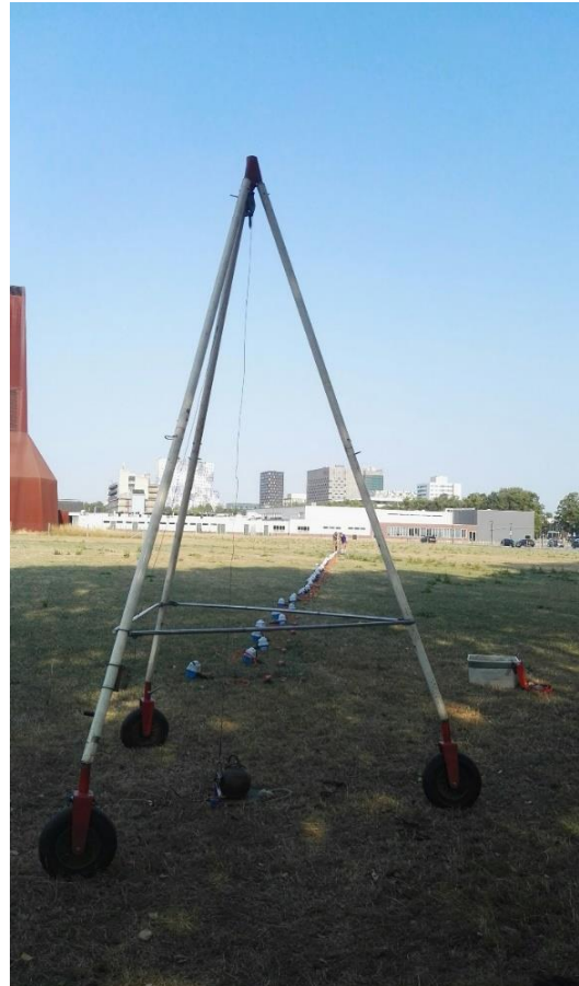
Figure 8. Field data acquisition design with the drop weight in front of the linear array.
