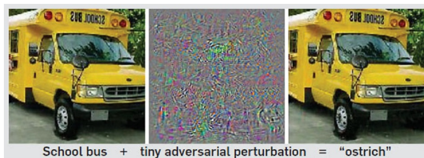
Figure 31: A convolutional neural network is shown to be easily influenced by a specific perturbation, figure from [Sze+13].
