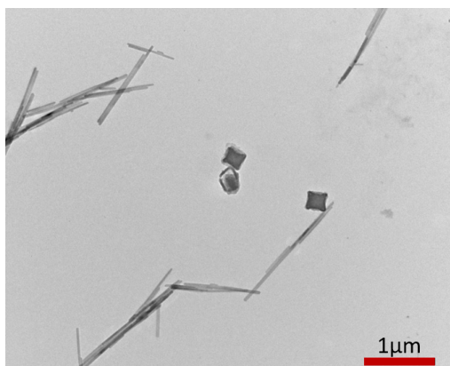
Figure 5.3: Goethite ( \alpha\text{-FeOOH} ) nanowires grown as an intermediate during the synthesis of hematite cubes.
