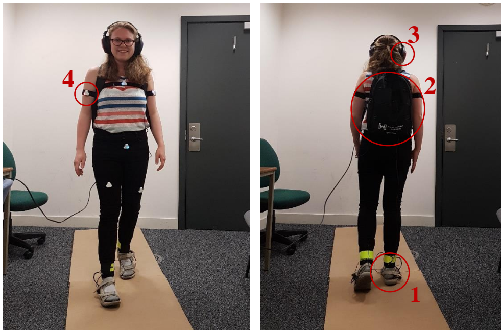
Figure 1: Equipment during the two walking phases. Participants wore strap-sandals with attached microphones (1), a small backpack containing a pre-amplifier and an equalizer (2), and headphones through which participants heard their modified footstep sounds (3). Black rubber bands with one of six Notch movement sensors (white triangles) each (4) were attached to the upper arms, chest, hip, and thighs.
