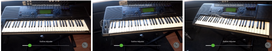
Figure 2.23: The output of Vuforia's Model Target pose detection from a guideview and subsequent tracking of the pose shows decent timing performance but poor accuracy for a musical keyboard use case. Notice how the tracked digital white keyboard overlay does not accurately match the musical keyboard in the camera feed.
