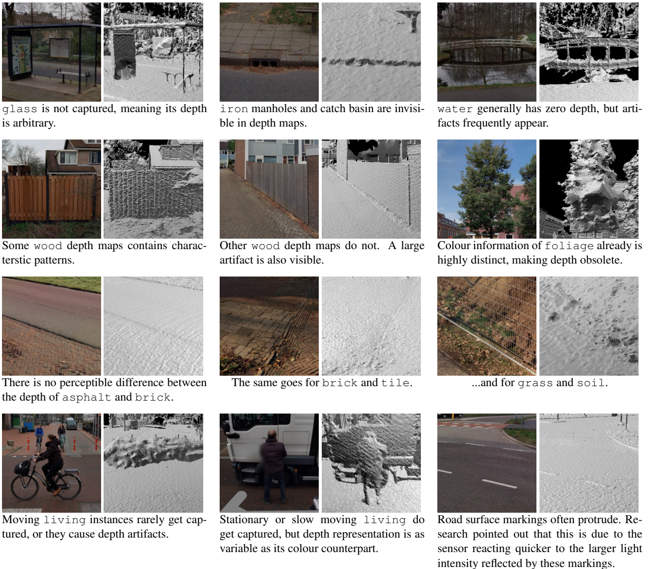
Figure 49: A compilation of materials and examples where depth is either worthless or adds noise and confusion. These examples are not incidental, but appear frequently.
