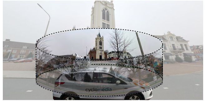
(b) Panoramic cameras mounted on top of the car capture 360° cylindrical photos, referred to as cycloramas.
