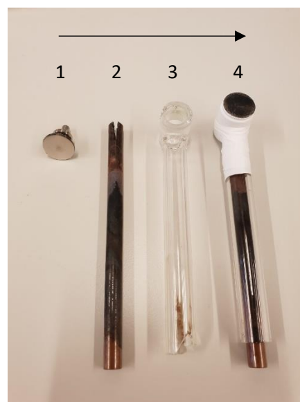
Figure 9. 1) titanium stub 2) copper rod 3) glass tube 4) Final electrode covered with Teflon tape
