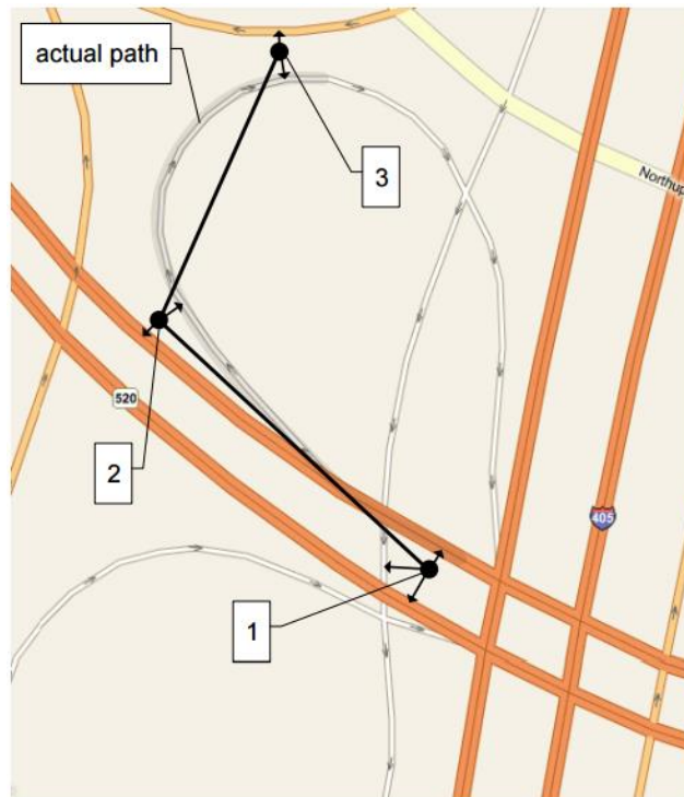
Figure 3.6: An example of choosing the logical route with a HMM (Newson & Krumm, 2009, p. 1)
