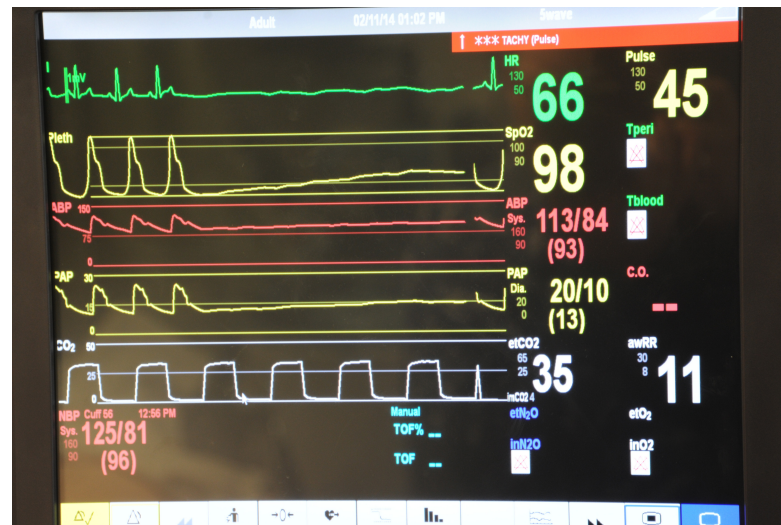
Figure 1.1: A patient monitor that shows a number of vital signs. Physicians and nurses use the vital signs to assess the condition of the patient. Furthermore, the monitor can alarm the caregivers if a vital sign moves outside a predefined range.
