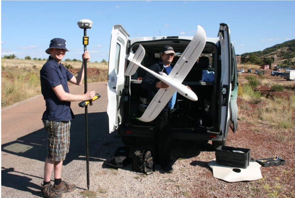
Figure 9, Fieldwork equipment; The RTK GPS, The raptor drone, the black dot on the front of the bottom side of the drone is a whole which behind which the lens of the camera is situated. One of the GCP markers can be seen underneath the black box.
